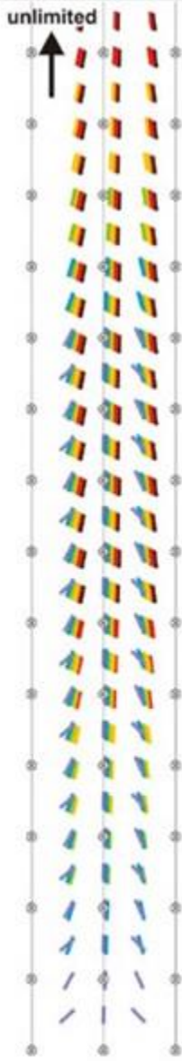
D POLE-DIPOLE OFF-LINE ARRAY a=200m to n=14 420 data, essentially uni-directional
